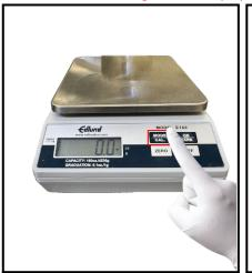
**Step 1:** Select the desired measuring unit by pressing the "Mode/Cal" button. (oz, g)
